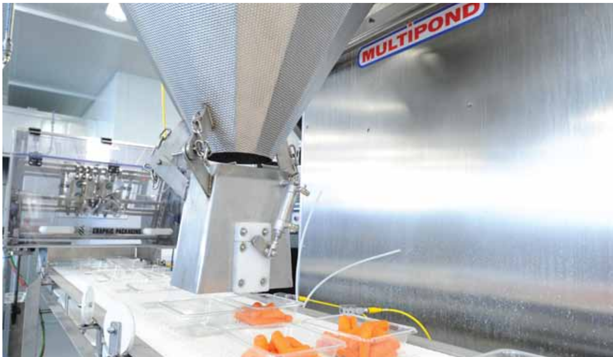
After a Graphics Packaging International denester places trays onto a conveyor, fresh-cut carrots are placed into the trays by a Multipond 12-head weigher installed by Abbey Packaging Equipment.
