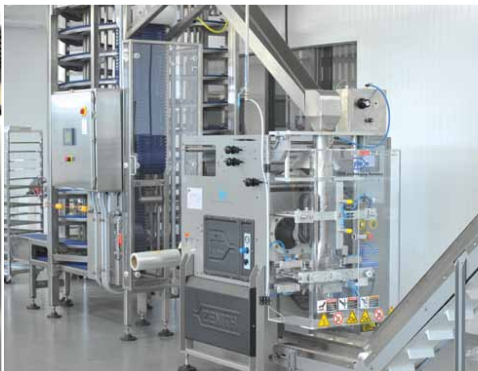
After cooling on a Tri-Mach spiral conveyor, freshly-baked goods are packed via a vertical form/fill/seal Zenith bagger from PFM Packaging Machinery.
