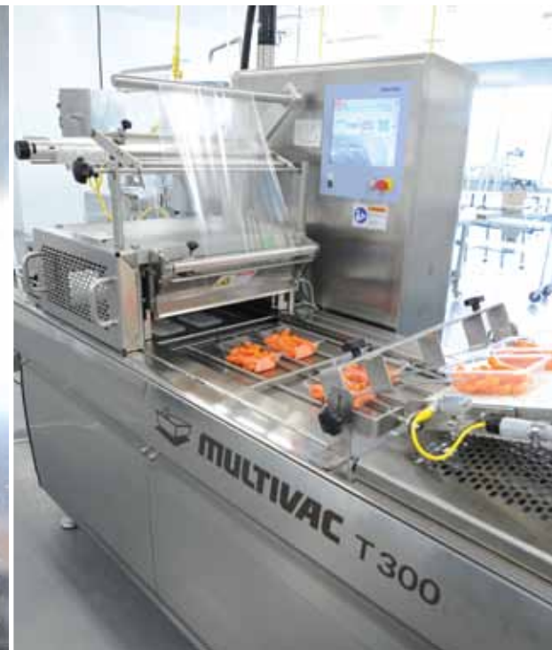
A compact, fully-automatic Multivac T300 tray-sealer combines innovative machine technology with a hygienic design to provide IFPT students with an excellent learning platform to hone their food process operating skills.
