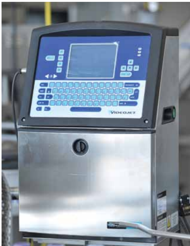
A Videojet 1220 small-character inkjet printer used to print lot and best-before codes onto bottling line containers.
