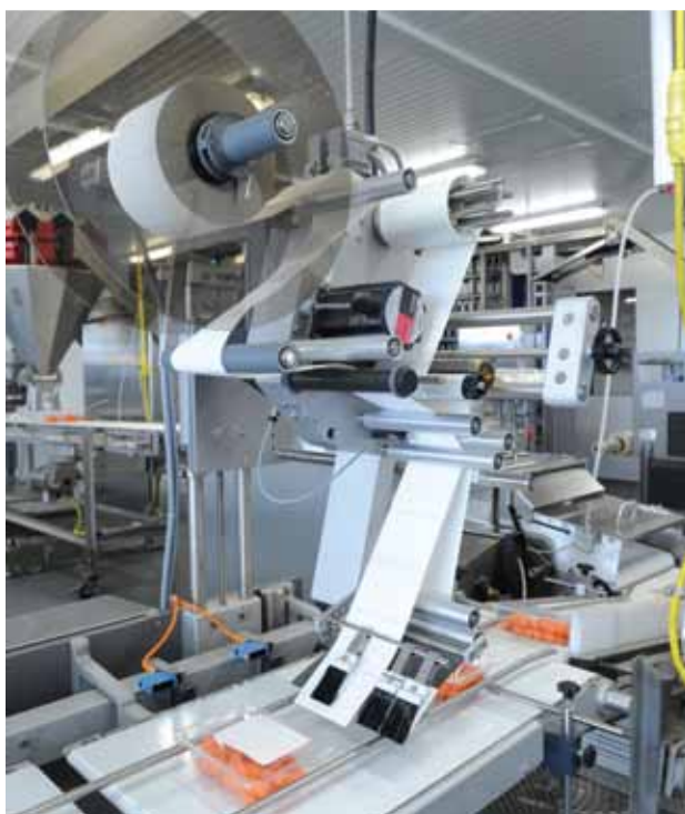
A Multivac MR 6411 labeler applies adhesive labels onto tray of carrots on the fresh-vegetable packaging line.
