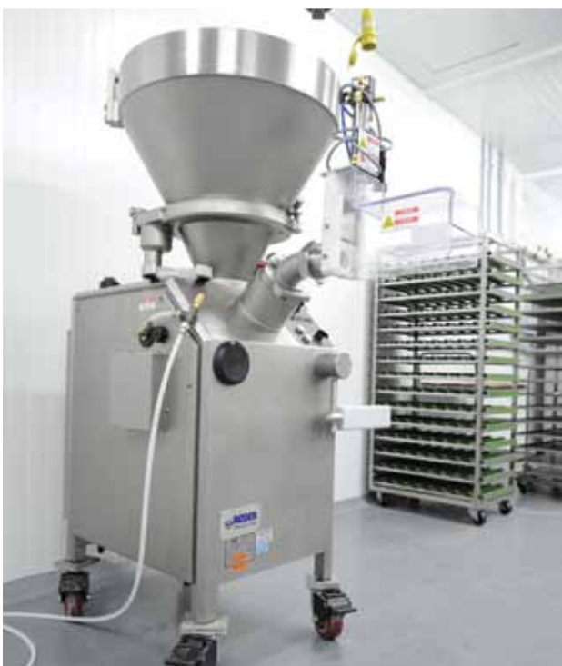
A Vemag PC878 portion controller from Reiser is used by IFPT students to prepare the fresh-baked goods for packaging.
