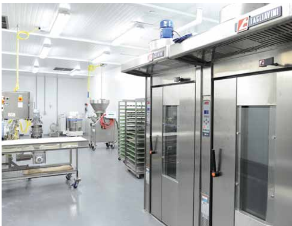
A pair of high-quality Tagliavini Rotovent model ovens and proofers/retarders designed for compact size, versatility and energy savings are employed in the IFPT's bakery.
