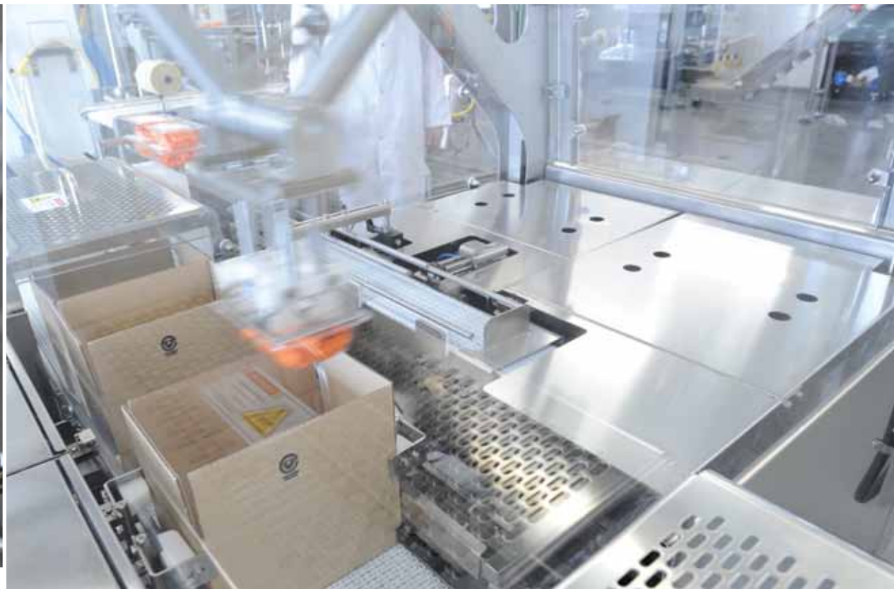
The Multivac H100 case-packer uses pick-and-place robotics to pack finished trays into corrugated cartons.
