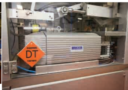
Distributed in Canada by R.E. Morrison, a high-performance Becker vacuum pump is incorporated into the Bosch twin-tube bagging machine to ensure precise air flow and distribution during the bagmaking process.
