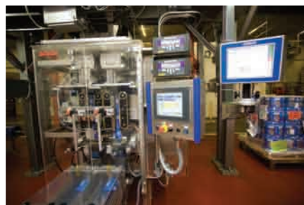
Two Markem-Imaje model SmartDate 5 small-character inkjet coding systems, positioned just above the Bosch bagger’s control panel, are used to apply date and production codes onto all the flexible plastic pouches of cookies exiting the bagging machine.
