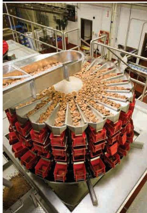
A high-performance Multipond multibucket scale dispenses perfectly measured deposits of freshly-made cookies into their proper buckets to feed the Bosch twin-tube from-fill-seal bagging machine directly below it on the floor level.
